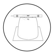
5. Place the bath upside down on a clean, smooth surface to protect the bathtub. Adjust the legs of the bath so they protrude 1/8 inch from the base of the bath.
