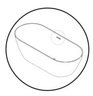
3. Install the exposed overflow plate. Refer to plan 3 b. of the bath drain at the bottom of the manual.
