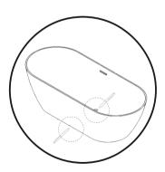
1. Clean, level and prepare the floor for installation. Place the tub in the appropriate location on the floor and trace the outline of the tub using a pencil or a marker. Then mark the location of the drain on the ground.
