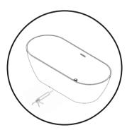
10. Fill the bathtub with water to the overflow, then empty it while inspecting the drain fittings located under the floor to check for potential water leaks.
