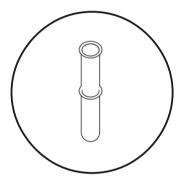
6. Attach the 1 1/2 inch female pipe thread to the 1 1/2 inch male tub drain (female pipe not included).
