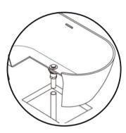
9. Carefully place the bathtub and connect the drain to the plumbing (previously installed). Complete the installation of the mounting piece.
