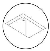
4. Before drilling a hole in the floor for the drain pipe, make sure there is nothing underneath (pipes, floor joints, heating ducts, electrical wires).
