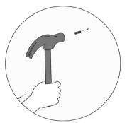
4. Insert screw anchor into the holes.
