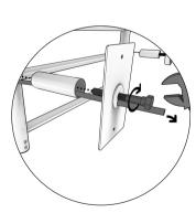
8. Pass the supply cable through the tube provided for this purpose and pass the wire through the plate. Rivet the base onto the fixing screw.
