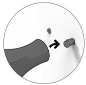
4. Insert screw anchor into the holes.
