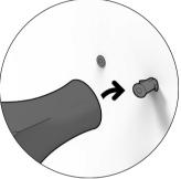
3. Insert screw anchor into the holes.
