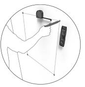
**1**. Identify the location of the holes needed to screw the product on the wall.
