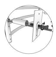
6. Pass the supply cable through the tube provided for this purpose and pass the wire through the plate. Rivet the base onto the nut with the fixing screw.
