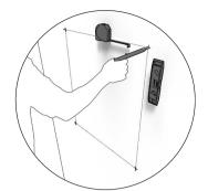
1. Identify the location of the holes needed to screw the product on the wall.
