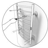
9. Install the base with the screws.
