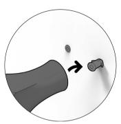
3. Insert screw anchor into the holes.
