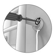
5. Install the base with the screw.
