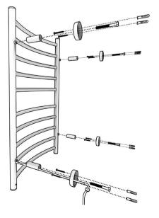
4. Rivet the base onto the nut with the fixing screw.
