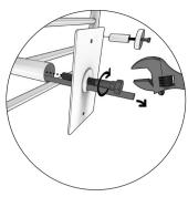
6. Remove the tube already present on the towel warmer and replace it with the tube available in the box provided for hardwired installation. Rivet the base onto the nut with the fixing screw.
