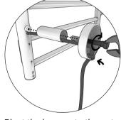
5. Rivet the base onto the nut with fixing screw.
