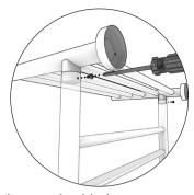
1. Slide the tray into the upper tubes and secure it with the screws.
