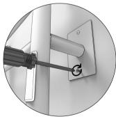
9. Connect the supply cable to the junction box and fix the plate onto the junction box.
