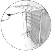
10. Install the base with the screws.
