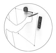
2. Identify the location of the holes needed to screw the product on the wall.
