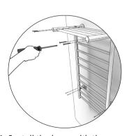
6. Install the base with the screw.
