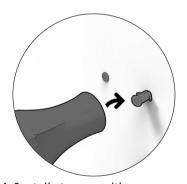
4. Install stopper with screw on the wall.
