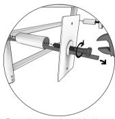
6. Pass the supply cable through the tube provided for this purpose and pass the wire through the plate. Rivet the base onto the fixing screw.
