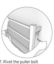
7. Rivet the puller bolt with the fixed stopper through allen key.
