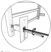
6. Cut the supply cable. Make sure you keep enough wire to go through the tube and to plug into the junction box. Remove the already existing tube to replace it with the one provided in the box of the hardwire installation.
