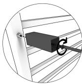
1. Rivet the base onto the nut with fixing screw.
