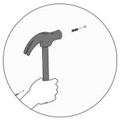
4. Insert screw anchor into the holes.
