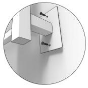
8. Connect the supply cable to the junction box and fix the plate onto the junction box.
