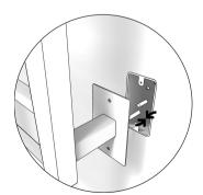
7. Pass the supply cable through the tube provided for this purpose and pass the wire through the plate.
