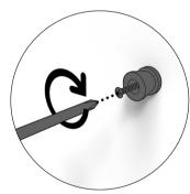
5. Install stopper with screw on the wall.
