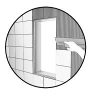
5. Apply your installation material and fix your tiles, marbles or stones directly on the shower wall. It is preferable that the tiles are symmetrical around the support structure.
