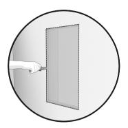
2. Trace the cutting line with a pencil, above the center line, cut a cavity in the wall panel along the drawn line. Make sure that the top and bottom lines are level.
