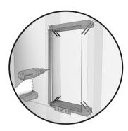
3. Level and secure the upper and lower support frame to the adjacent vertical studs.
