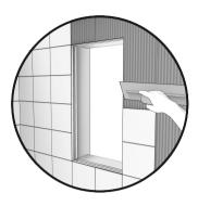
5. Apply your installation material and fix your tiles, marbles or stones directly on the shower wall. It is preferable that the tiles are symmetrical around the support structure.
