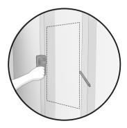
1. Locate and mark the center lines of the adjacent wall studs using a stud finder. Draw a level line between the two wall studs at the desired height to insert the niche.
