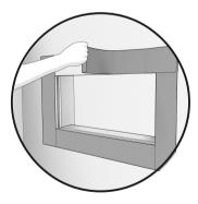
4. Install the waterproofing membrane to seal the support structure and the cavity (not included).
