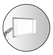
6. Apply a necessary layer of silicone around the back periphery of the flange of the niche to ensure watertightness.
