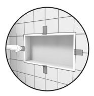
9. Add adhesive tape to hold the niche in place until the silicone has hardened.
