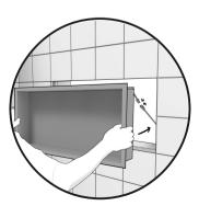
8. Insert the niche into the cavity and connect the niche connector to the 12 volt wire connector. Press firmly on the flange and make sure the niche is in place. It is recommended to seal the space between the flange and the tile.
