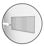
2. Trace the cutting line with a pencil, above the center line, cut a cavity in the wall panel along the drawn line. Make sure that the top and bottom lines are level.
