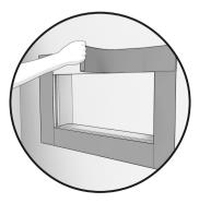
4. Install the waterproofing membrane to seal the support structure and the cavity (not included).
