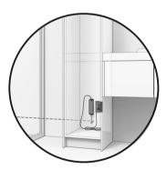
7. Install the supplied transformer to power the niche light. The transformer must remain accessible so you can provide a place to hide it.
