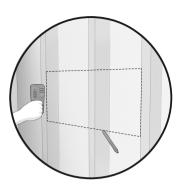
1. Locate and mark the center lines of the adjacent wall studs using a stud finder. Draw a level line between the two wall studs at the desired height to insert the niche.
