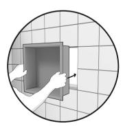
7. Insert the niche into the cavity. Press firmly on the flange and make sure that the niche is in place. It is recommended to seal the space between the flange and the tile.
