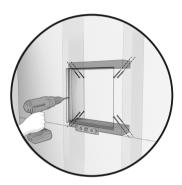
3. Level and secure the upper and lower support frame to the adjacent vertical studs.
