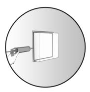
6. Apply a necessary layer of silicone around the back periphery of the flange of the niche to ensure watertightness.
