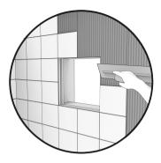
5. Apply your installation material and fix your tiles, marbles or stones directly on the shower wall. It is preferable that the tiles are symmetrical around the support structure.
