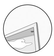
10. To activate or deactivate the light, wave your hand near the contactless switch located at the top right, inside the niche.
