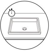
5. Let the putty dry for a few hours before connecting the water supply and drain pipes.
