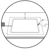
2. Trace the dimensions of the holes to be drilled in the counter. Measure the space required for the installation of the drain and faucet.
