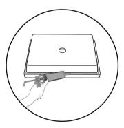
4. Apply plumber's putty along the inside edge under the washbasin. Place the washbasin in the desired location. Press firmly to spread the sealant and immediately wipe off the excess with a damp cloth.
