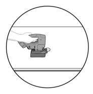
3. Cut the opening using a jigsaw. Use a soft cloth between the surface of the counter and the saw to not damage or scratch the counter.
