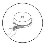
4. Apply plumber's putty along the inside edge under the washbasin. Place the washbasin in the desired location. Press firmly to spread the sealant and immediately wipe off the excess with a damp cloth.
