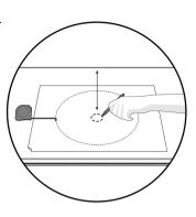
2. Trace the dimensions of the holes to be drilled in the counter. Measure the space required for the installation of the drain and faucet.
