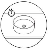
5. Let the putty dry for a few hours before connecting the water supply and drain pipes.
