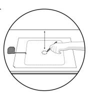
2. Trace the dimensions of the holes to be drilled in the counter. Measure the space required for the installation of the drain and faucet.
