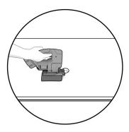
3. Cut the opening using a jigsaw. Use a soft cloth between the surface of the counter and the saw to not damage or scratch the counter.
