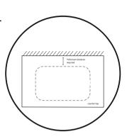
2. Trace the dimensions of the holes to be drilled in the counter. Measure the space required for the installation of the drain and faucets.
