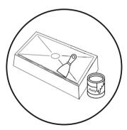
4. Apply plumber's putty along the inside edge. Place the washbasin in the desired location. Press firmly to spread the sealant and immediately wipe off the excess with a damp cloth.
